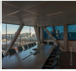
SageGlass® is the result of **25 years of Research and Development** and over **500 patents have been filed.** It is much more than a piece of glazing: it transforms buildings by making façades and glass roofs adaptive and intelligent. This active glass, unrivalled in terms of performance on the market, darkens and lightens electronically while constantly remaining transparent, to ensure **thermal and visual comfort** to the building's occupants, whatever the weather.
